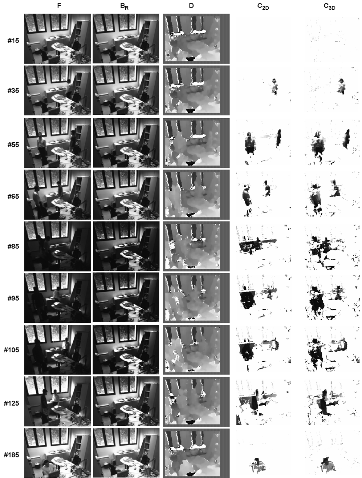
Figure 5. Experimental results on 9 frames of the Office stereo sequence using the disparity map provided by the SMP algorithm [3]. (First column) - Reference image F of the stereo pair. (Second column) Background model B_{2D} registered according to the specification given by the histogram of the frame F . (Third column) - Disparity map D computed by the SMP algorithm. (Fourth column) - Change mask C_{2D} provided by the proposed 2D Output approach. (Fifth column) - Change mask C_{3D} provided by the proposed 3D Output approach.
