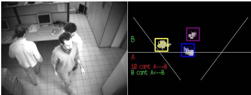
Fig. 10. Frame 0189 of the "Count" stereo sequence. (Left) Original left image. (Right) plan-view map with the tracked people and statistics about the crossings in the two directions.
